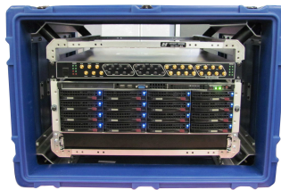
Portable Shipping Case with Shock-Mounted Racks & wheels
