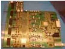
22 Layer DSP & 10 Gigabit Network Interface Board
