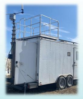
D-TA Systems MFEL-1000 is a highly effective, low-cost tool capable of EMCON monitoring during military exercises. The MFEL-1000 is capable of sensing from 2-18 GHz at 500MHz IBW, can be easily installed on an ATV, van, container or trailer as shown on the left.
