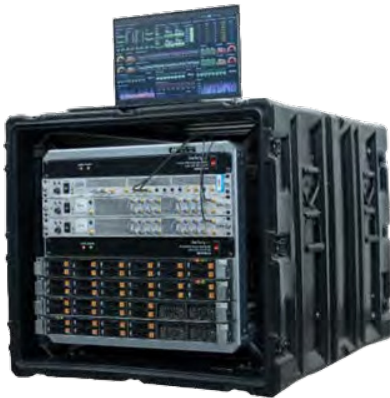
A 64-channel streaming I/Q based OTHR stimulator in a portable carrying case for ease of Rx testing.
