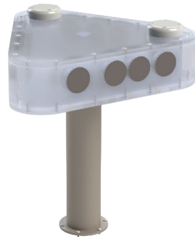
Soldier-Portable MFEL With linear antenna array (4 spirals in each of 3 sides for 360 ° FOV on 1° DF accuracy)
