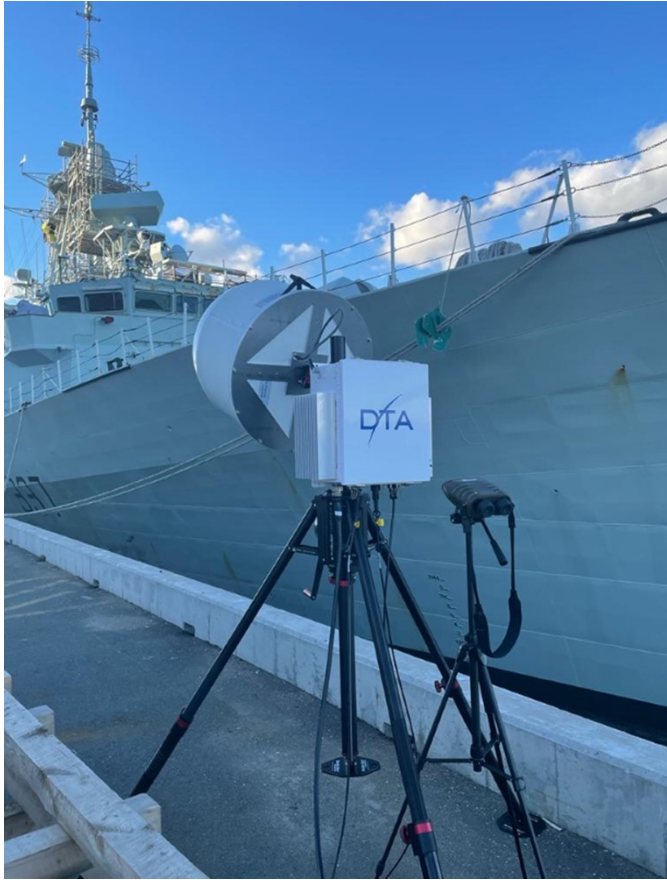
Dockside testing of ship's ESM receiver using the PETS system.
